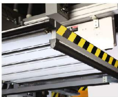
Anti-collision Anti-pressure Equipment in Work Table (3 Safety Trim Strips)
